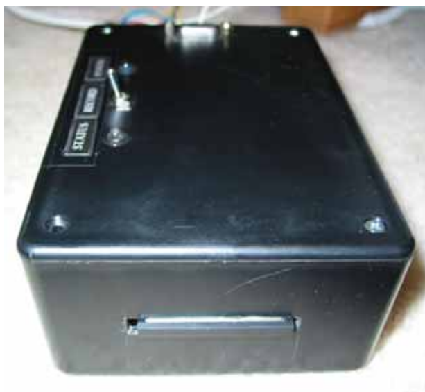
Figure 25. Assembled TND Prototype Multiplexer and Computer Showing CompactFlash Card
