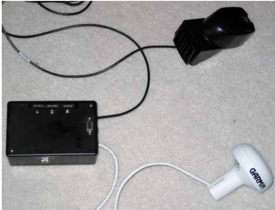
Figure 24. The Complete TND Hardware, including Multiplexer Box, Garmin WAAS GPS, and Temperature and Depth transducers in One Airmar Unit
